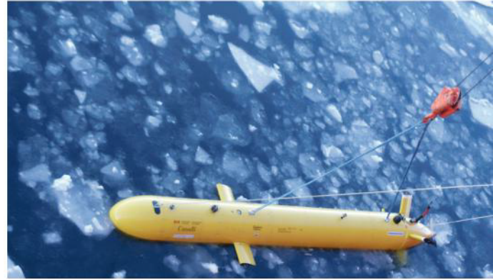
Autonomous underwater vehicle being launched from the CCGS Louis S. St-Laurent in 2011
