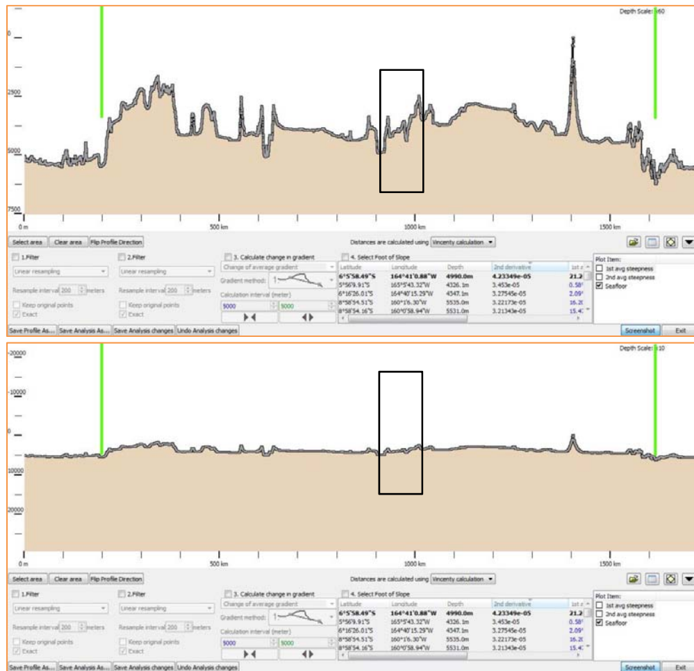
Figure 18b: Examination of morphological continuity of the continental slope through bathymetric profiles at scales of 1:60 and 1:10 across the DIT along “bridges” located between the North Plateau, the Western Plateaus and the High Plateau using MBES data only.
