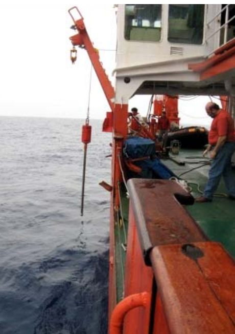
Sampling with gravity corer aboard the R/V Hespérides
