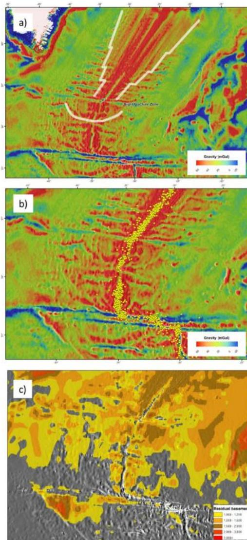
Figure 12. (a) The southern boundary of the V-shaped area (concave white band south of the Bight Fracture Zone), together with the western and eastern boundaries. Marine gravity in the background. (b) Marine gravity and earthquakes. (c) Residual basement depth [Main Body].
