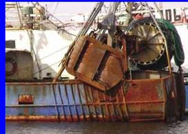
**Trawling gear is extremely robust – doors can be up to 5 tons each**
