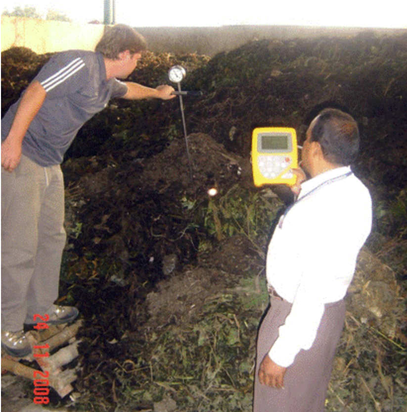
Regular Oxygen Monitoring
