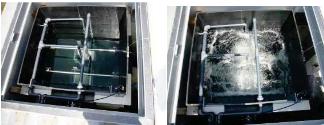
Figure 3. The membrane bioreactor with membrane units visible underwater (left), the membrane bioreactor aerated (right)
