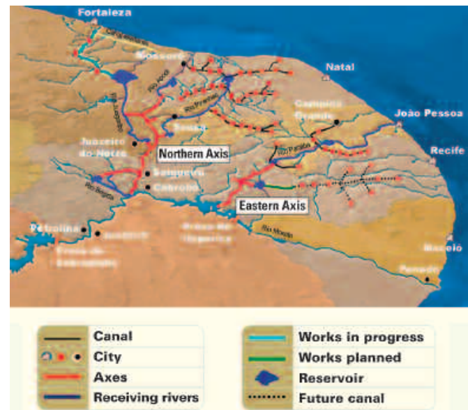
Fig. 6. Diagram of the San Francisco river diversion. PISF Project. National Water Agency (Brazil).
