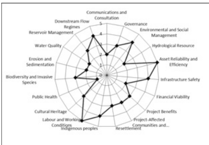
Figure (1): Sustainability Profile: For each sustainability topic, performance is scored from 1 to 5, with 5 being 'proven best practice'. The results are presented in an easy-to-read profile as shown in this figure.
